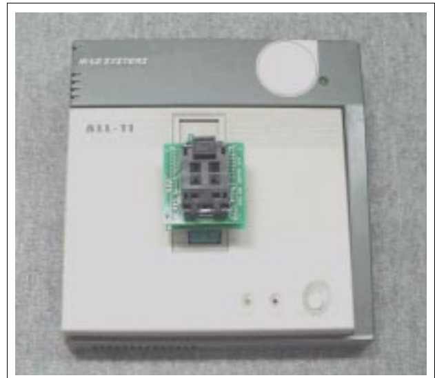
Figure 9-2 ALL-11 Programmer with adapter
